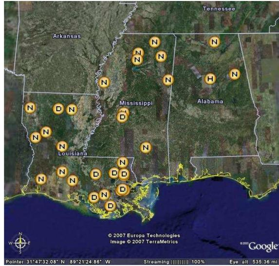
**Fig. 7.** Impact degree of network-service disruption. (N):  $T_{fail} < T_{fail}^*$ , (H):  $T_{fail}^* < T_{fail} < 24$  hours, and (D):  $T_{fail} \geq 24$  hours.
