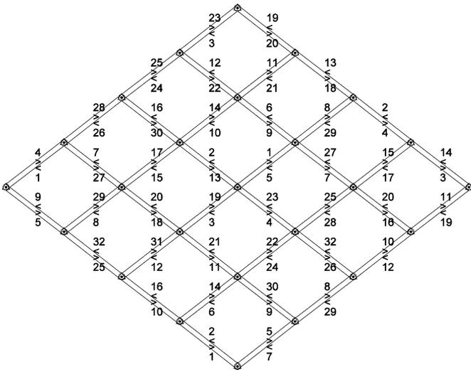
Fig. 10. Time slot allocation of spatial time division multiple access.
