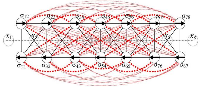
Fig. 1. Spatial dependency graph of link activities  $\sigma$  given a set of node positions  $\mathbf{X}$ .
