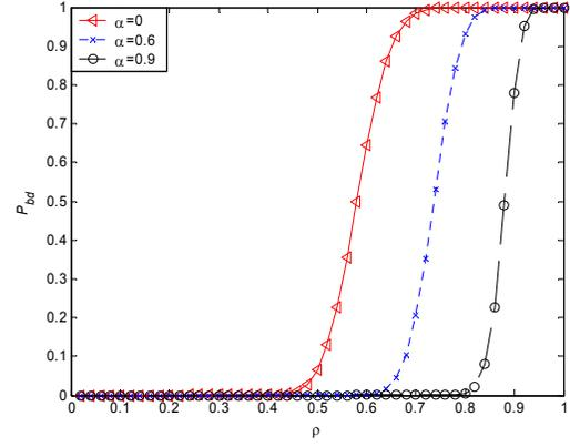
Fig. 7. Load ( $\rho$ ) vs. blocking probability ( $P_{bd}$ ):  $F=120$ ,  $H=5$ ,  $L=3$ ,  $\alpha=0, 0.6, 0.9$ ,  $P_l=0.2$ .
