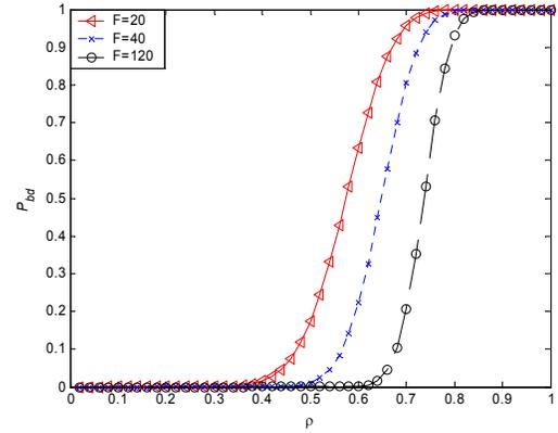
Fig. 8. Load ( $\rho$ ) vs. blocking Probability ( $P_{bd}$ ):  $F=20, 40, 120$ ,  $H=5$ ,  $L=3$ ,  $\alpha=0.6$ ,  $P_l=0.2$ .
