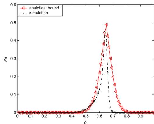
Fig. 10. Analytical bound and simulated  $P_e$ :  $F=40$ ,  $H=5, L=3, \alpha=0.6, P_l=0.2$ .
